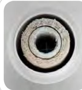
**EN.** Typical condition of the filter after transferring 30,000 litres.
