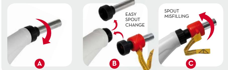
**EN.** Safety is guaranteed by the break-away system. In the event that a vehicle accidentally drives away with the nozzle still in the tank, the spout is designed to detach from the nozzle. This system also allows for a quick repair by merely fitting a new spout onto the nozzle.
